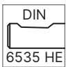
Mango WHISTLE NOTCH MD HM WHISTLE NOTCH Shank Queue WHISTLE NOTCH carbure
