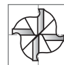
4-5 Z= 4-5 Dientes. Corte al Centro 4-5 Z= 4-5 Flutes. Center Cutting 4-5 Z= 4-5 Dents. Coupe au centre
